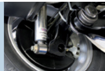
Stainless steel shock absorber, that we developed, on the rear axle of a W111
