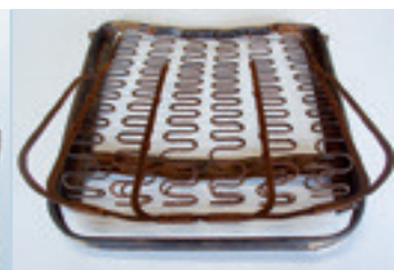
Original, unrestored W111 seat underframe
